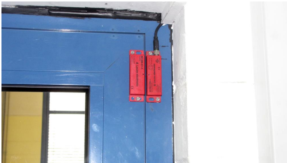
Figure 6. Behind the doors, MC300 magnetically coded sensor perform position monitoring and thereby ensure the required Performance Level.
